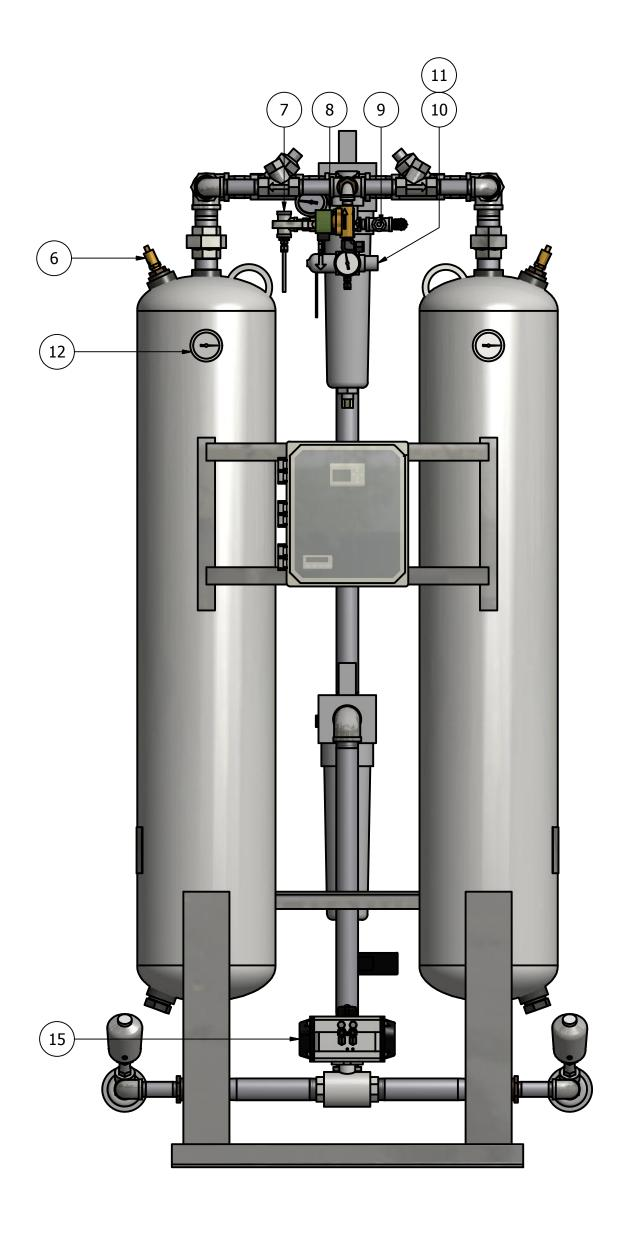
PRESSURE REGULATOR, PURGE PRESSURE GAUGE, PURGE 3 CHECK VALVE, OUTLET 4 PARTICULATE AFTER-FILTER 5 RELIEF VALVE, TANK 6 DEW POINT MONITOR (OPTIONAL) SOLENOID VALVE, REPRESS 8 MOISTURE INDICATOR 9 PRESSURE REGULATOR, CONTROL 10 PRESSURE GAUGE, CONTROL 11 PRESSURE GAUGE, TANK 12 13 COALESCER PRE-FILTER TIMED DRAIN 14 3 WAY BALL VALVE, INLET 15 ANGLE BODY VALVE, EXHAUST 16 MUFFLER, EXHAUST 17 MANUAL BALL VALVE, BYPASS 18 330 LBS DESICCANT
